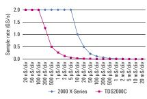
40x the memory allows you to keep sample rates higher on longer time/div settings
